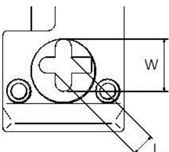
\* STD L = 8.6 mm MIN VERSCHLEISS L = 10.6 mm
