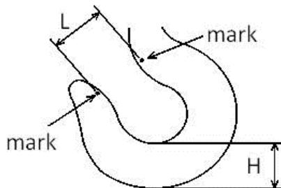
\* STD L = 8.6 mm MIN VERSCHLEISS L = 10.6 mm
