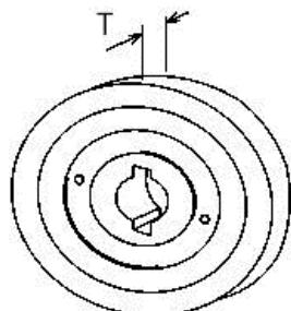
STD D = 8 mm MAXVERSCHLEISS B = 7.3 mm
