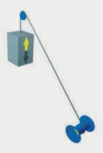
A **traversing winch** can be used to move a load in two directions on a level. You can therefore move a carriage forwards and backwards for example. The cable drum is designed for two cables, is scored and winds in only one layer.
